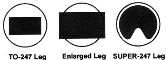
Fig. 11.7 Reduction of the electrical resistance of contact leads in a TO package [Swa00]
