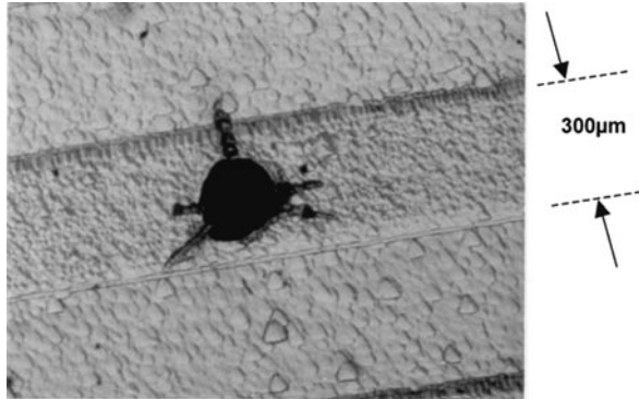
Fig. 12.26 GTO thyristor failed by exceeding the maximum turn-off current. Molten channel, created by a current filament in the middle of the cathode finger
